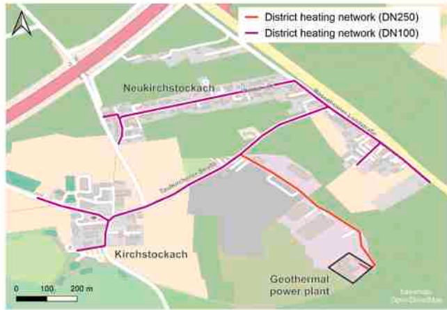
Fig. 2. Hypothetical DHN in Kirchstockach showing the main (diameter DN 250 mm) and intermediate heating grid (diameter DN 100 mm) with an overall length of 4,000 m. Exact locations of the smaller connection grid are not shown, but estimated per heat customer (see Table 4).
