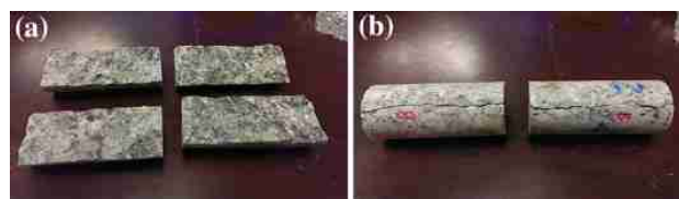
Fig. 3 Example of overcored specimen a open and b closed
